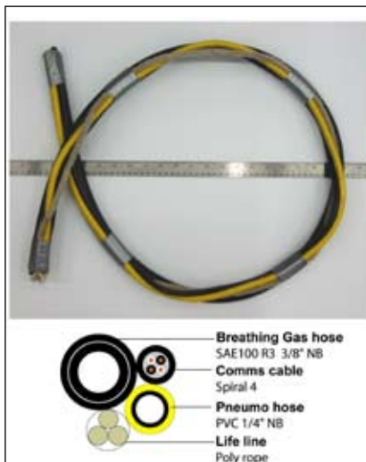
Typical 3 part taped umbilical construction, note the cross hovers and uneven bending when coiled (even on a relatively large radius of 8")
